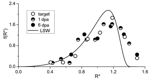
**Fig. 9.** Precipitate size distributions  $f(R^*)$  for the annealed alloy Fe-30%Cr-5%Al irradiated to various irradiation doses  $\phi$  at  $T = 710$  K and  $\kappa = 10^{-6}$  dpa/s
