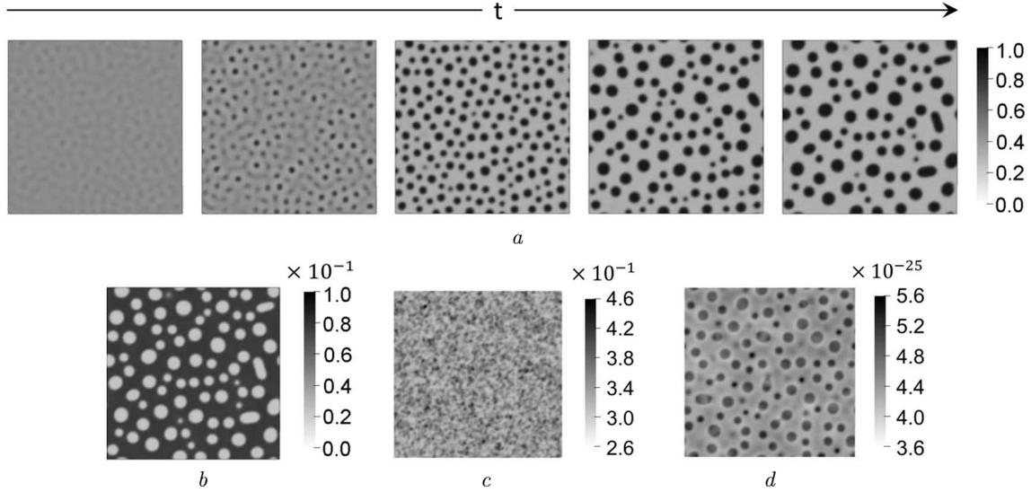
**Fig. 4.** Evolution of the chromium concentration field in the Fe-30%Cr-5%Al alloy (a). Distributions of aluminum concentration (b), vacancy concentration (c), and interstitial concentration in the annealed specimen (d)
