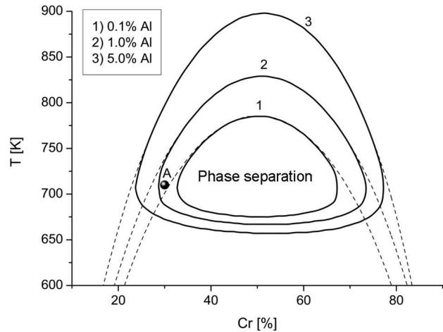
**Fig. 1.** Phase diagrams for Fe–Cr–Al alloys with various aluminum contents. Dashed curves correspond to non-irradiated systems. Solid curves correspond to irradiated systems at  $\mathcal{K} = 10^{-6}$  dpa/s
