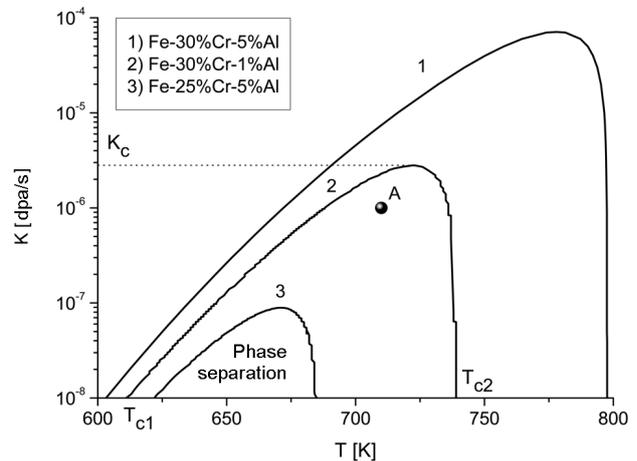
**Fig. 3.** Phase diagrams for various Fe–Cr–Al alloys
