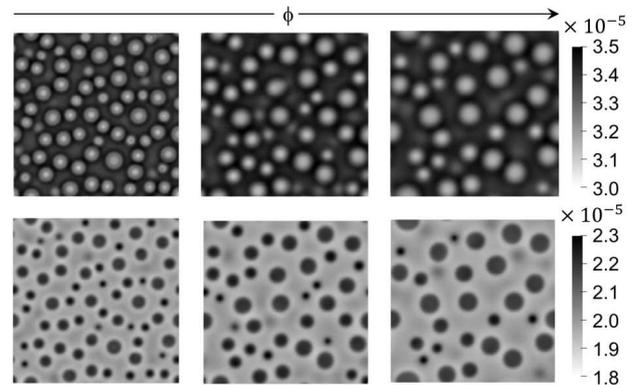
**Fig. 6.** Typical evolution of the spatial distributions of non-equilibrium vacancies (upper panels) and interstitial atoms (lower panels) in the Fe-30%Cr-5%Al alloy under irradiation at the dose rate  $\mathcal{K} = 10^{-6}$  dpa/s and the temperature  $T = 710$  K
