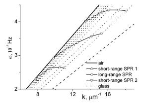
$\pmb{Fig. 5.}$  Dispersion characteristics  $\omega(k)$  of the SPR in an Au film with  $d=50~\mathrm{nm}$
