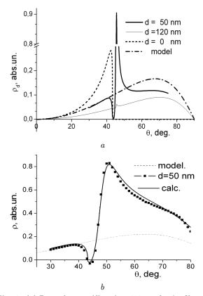
Fig. 2. (a) Dependences  $\rho(\theta)$  at  $\lambda=632$  nm for Au films of various thicknesses and the model non-resonant component for a film with d=50 nm. (b) The same as in panel (b) but for a film with d=50 nm at  $\lambda=550$  nm: experimental and theoretical dependences, and its non-resonant component (dashed curve)
