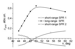
Fig. 6. Dependences of the amplitudes of Gaussian-like components that approximate the normalized  $\rho_{\rm SPR}$  on the light incidence angle
