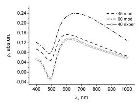
Fig. 3. Spectral dependences of the non-resonance component of the parameter  $\rho(\theta)$  obtained at the measurement at the incidence angle  $\theta=40^{\circ}$  and the model curves calculated for the angles  $\theta=45^{\circ}$  and  $60^{\circ}$
