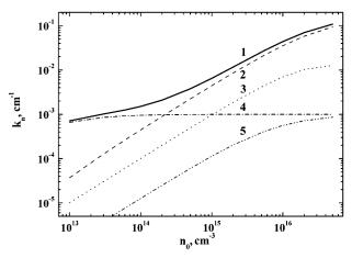
Fig. 4. Calculated dependences  $k_n(n_0)$  for n-Si irradiated with 1-MeV electrons: cumulative contribution (1) and contributions of components VP (2), VO (3),  $V_2^{-/0}$  (4), and  $V_2^{--/-}$  (5)
