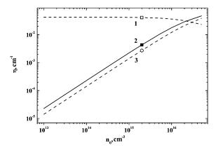
Fig. 6. Dependences of the formation efficiency  $\eta$  on the concentration  $n_0$  for main compensating radiation-induced defects in  $n\text{-Si}\langle \mathrm{Sn}\rangle$  with  $[\mathrm{Sn}] = 2 \times 10^{17}$  cm<sup>-3</sup> (curve 1 for SnV and curve 3 for VP) and reference n-Si (curve 2 for VP). Solid curves correspond to the results of calculation by formulas (4) and (5), and points to experimental data
