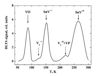
Fig. 2. DLTS spectrum for  $n\text{-Si}\langle \mathrm{Sn}\rangle$  irradiated with 1-MeV electrons ( $\Phi_e = 1 \times 10^{16} \ \mathrm{cm}^{-2}$ )
