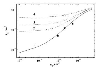
Fig. 3. Dependences  $k_n(n_0)$  for n-Si with various Sn concentrations of 0 (1),  $2 \times 10^{16}$  (2),  $5 \times 10^{16}$  (3), and  $2 \times 10^{17}$  cm<sup>-3</sup> irradiated with 1-MeV electrons. Solid curves correspond to calculation results, and points to experimental data
