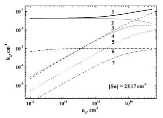
Fig. 5. Calculated dependences  $k_n(n_0)$  for  $n\text{-Si}\langle \mathrm{Sn}\rangle$  irradiated with 1-MeV electrons: cumulative contribution (1) and contributions of components  $\mathrm{SnV}^{-/0}$  (2), VP (3),  $\mathrm{SnV}^{--/-}$  (4), VO (5),  $\mathrm{V_2^{-/0}}$  (6), and  $\mathrm{V_2^{--/-}}$  (7)
