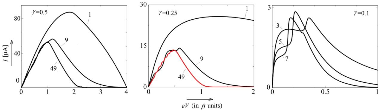
**Fig. 3.** I–V characteristics of contacts of lengths  $\mathcal{N} = 1, 9, 49$  (left and middle panels) and  $\mathcal{N} = 3, 5, 7$  (right panel) for different values of  $\gamma$  and  $\beta^{\text{cont}} = \gamma$ . The curve for  $N = 49$  in the middle panel is marked with red color for clarity
