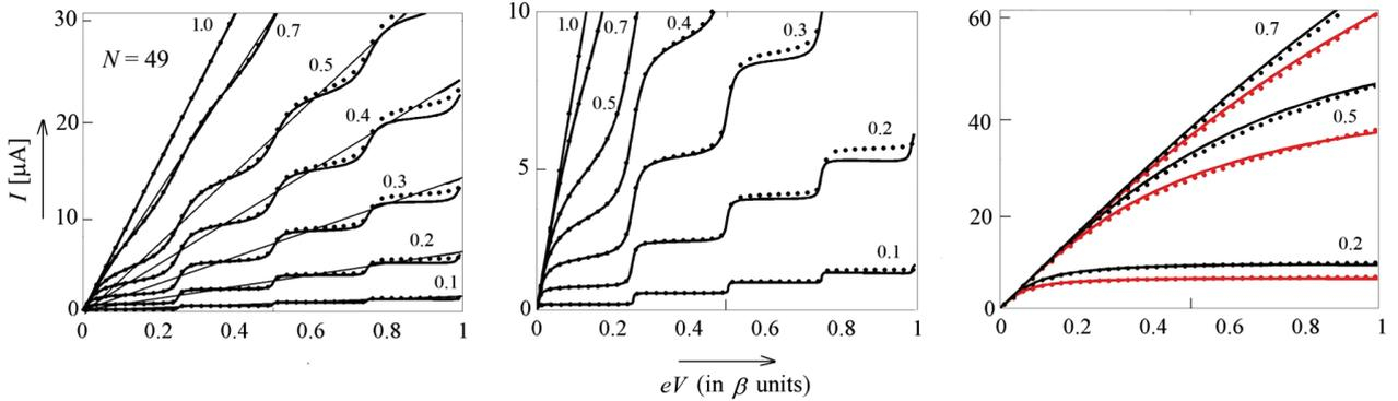
**Fig. 4.** Left panel: The exact dependence  $I(eV)$  given by Eq. (21) is depicted by solid lines while its approximation (22) is displayed by dotted lines calculated for  $\mathcal{N} = 49$ ,  $\beta^{\text{cont}} = 1$  and  $\gamma = 0.1, 0.2, 0.3, 0.4, 0.5, 0.7$ , and  $1.0$ . Central panel: Enlarged dependences shown in the left panel. Right panel: The same dependences for  $N = 3$  (black),  $N = 5$  (red), and  $\gamma = 0.2, 0.5$ , and  $0.7$ .
