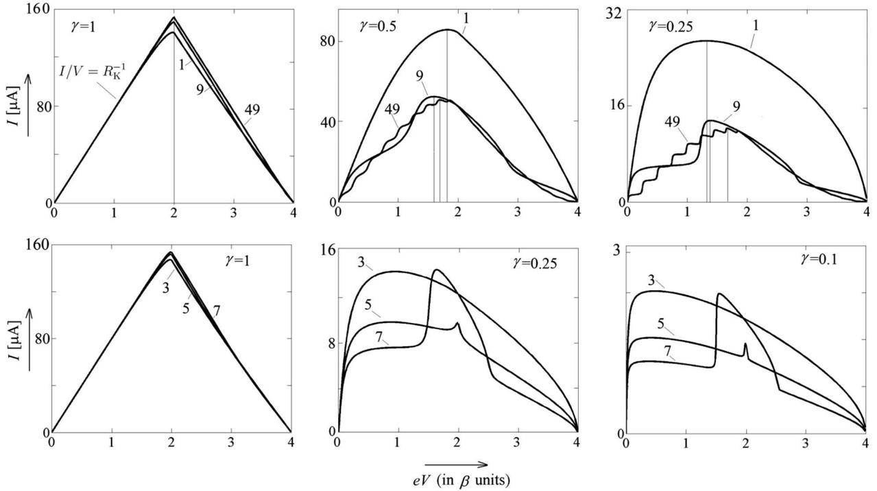
**Fig. 2.** I–V characteristics of contacts of lengths  $\mathcal{N} = 1, 9, 49$  (top panel row) and  $\mathcal{N} = 3, 5, 7$  (bottom panel row) for different values of  $\gamma$  and  $\beta^{\text{cont}} = 1$ . The left side of perfect isosceles triangle ( $\mathcal{N} = 49, \gamma = 1$ ) corresponds to the volt-ampere characteristic  $I = \frac{2e^2}{h}V, h/(2e^2) = 12.9k\Omega$
