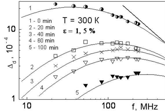
Fig. 1. Frequency dependence of the dislocation resonance absorption of ultrasound in LiF crystals preliminarily deformed to  $\varepsilon = 1.5\%$  at  $T = 300$  K at various irradiation times  $t$ , min: 1 – 0; 2 – 20; 3 – 40; 4 – 60; 5 – 100
