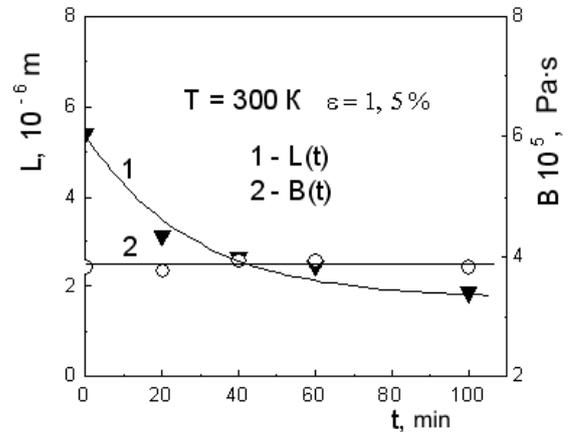
Fig. 3. Dislocation segment length (1) and the dislocation damping coefficient (2) as functions of the irradiation time of LiF crystals
