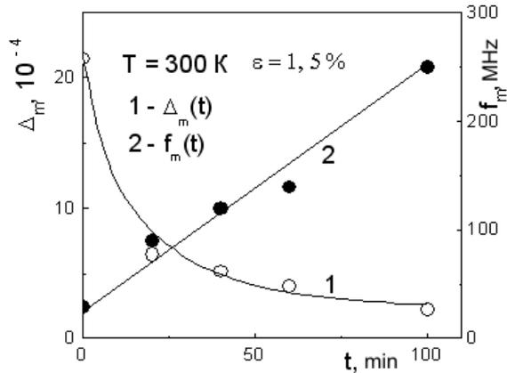
Fig. 2. Decrement  $\Delta_m$  (1) and the resonance frequency  $f_m$  (2) as functions of the irradiation time of LiF crystals
