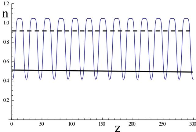
Fig. 3. Spatial dependence of the exciton density at various values of the pumping:  $G = 0.0056$  for the continuous line,  $G = 0.007$  for the periodic line, and  $G = 0.00924$  for the dashed line.  $D_1 = 0.03$ ,  $b = -1.9$
