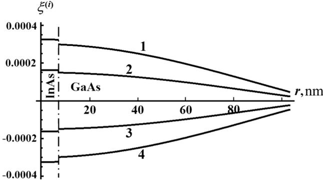
Fig. 3. Spatial distributions of the uniform deformations  $\xi(r)$  in the QD and matrix materials at various time moments,  $\omega t = \frac{\pi}{2}$  (1),  $\frac{\pi}{6}$  (2),  $\frac{7\pi}{6}$  (3), and  $\frac{3\pi}{2}$  (4)
