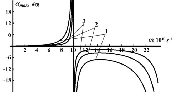
Fig. 4. Dependences of the deviation angle amplitude of emission from an InAs/GaAs heterolaser with InAs QDs on the acoustic wave frequency for various QD dimensions:  $R_0 = 3$  (1), 6 (2), and 9 nm (3)
