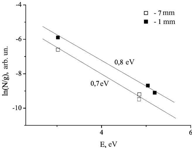
Fig. 4. Electron temperature in the CuInSe<sub>2</sub> laser plasma determined based on the excited-state population distribution of indium atoms
