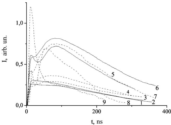
Fig. 2. Radiation oscillograms of the  $\text{CuInSe}_2$ -based laser erosion plasma at 1 mm from the target: 1 – 521.8 nm Cu I; 2 – 515.3 nm Cu I; 3 – 410.2 nm In I; 4 – 451.1 nm In I; 5 – 327.4 nm Cu I; 6 – 324.8 nm Cu I; 7 – 303.9 nm In I; 8 – 293.3 nm In I; 9 – 271 nm In I
