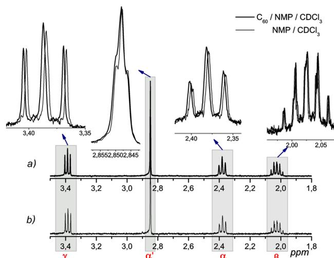
Fig. 1. NMR spectra of the initial NMP solution (a) and the solution NMP/C<sub>60</sub> (b)
