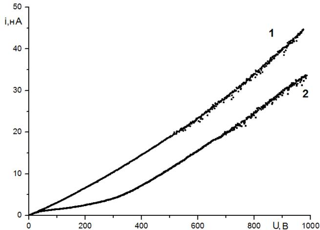
Fig. 3. Current-voltage dependences of the dark (1) and X-ray conductivities (2) of a single-crystal ZnSe specimen at room temperature
