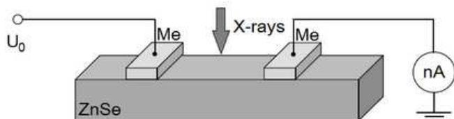
Fig. 1. Scheme of measurements of the X-ray conductivity
