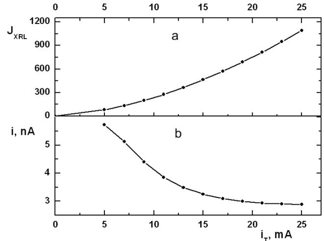
Fig. 4. Dependences of the XRL intensity (a) and the XRC current (b) on the X-ray radiation intensity (values of anodic current of an X-ray tube) at  $U_0 = 165$  V
