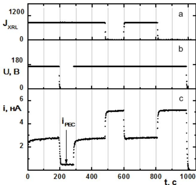
Fig. 2. Time dependence of the intensity of the X-ray luminescence band at 630 nm (a), supplied voltage  $U_0 = 165$  V (b), and the conductivity current (c) for a ZnSe specimen at room temperature
