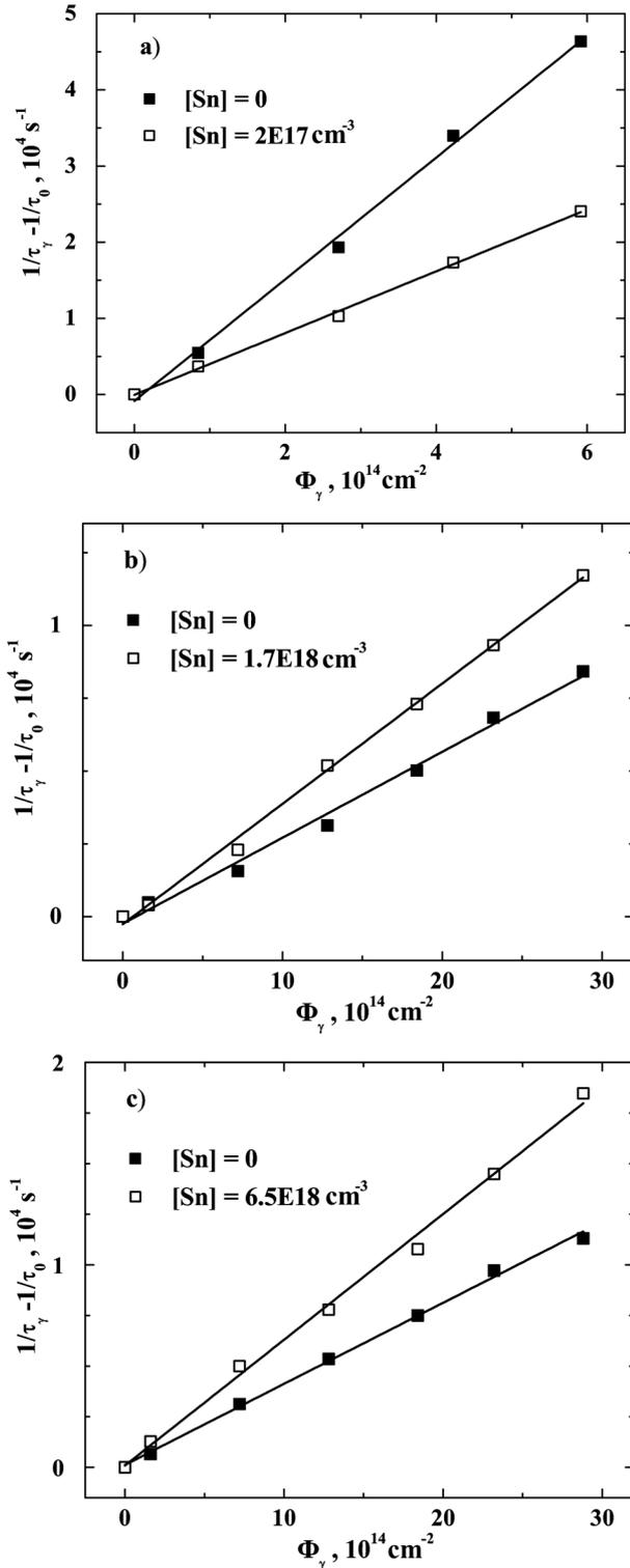
Fig. 1. Dependences of  $\Delta(1/\tau)$  on the dose of irradiation with  $\gamma$ -quanta of  $^{60}\text{Co}$  for Sn-doped  $n$ -Si samples. Symbols correspond to experimental data and curves show their linear approximations
