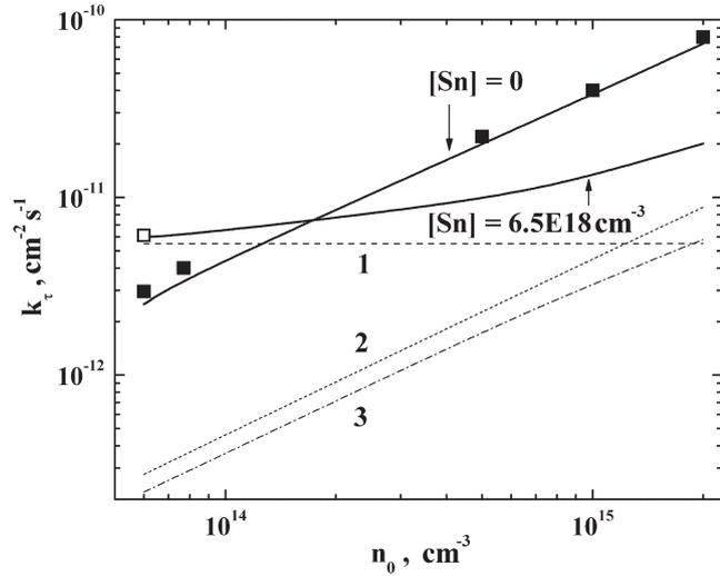
Fig. 2. Experimental (symbols) and calculated (solid curves) dependences of  $k_{\tau}$  on the free electron concentration for the  $\gamma$ -irradiated  $n$ -Si and  $n$ -Si(Sn-3) samples. Solid curves correspond to the VO contribution for  $n$ -Si and the cumulative contribution by the components  $\text{SnV}^{-/0}$  (1), VO (2), and  $\text{SnV}^{-/-}$  (3) for  $n$ -Si(Sn-3)
