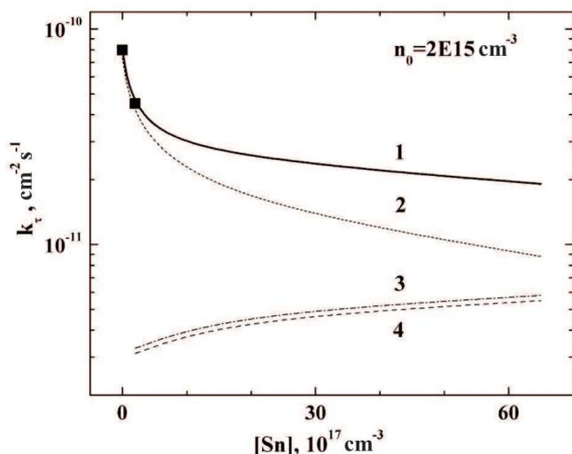
Fig. 3. Calculated dependence of  $k_{\tau}$  on the tin concentration for the  $\gamma$ -irradiated low-resistance  $n$ -Si(Sn-3) sample (1) and its components: VO (2),  $\text{SnV}^{--/}$  (3), and  $\text{SnV}^{-/0}$  (4). Points correspond to experimental data
