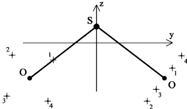
Arrangement of atoms in SO<sub>2</sub> molecule with respect to the coordinate axes. The symbols “+” to the left from the ordinate axis correspond to the consecutive, marked by figures, positions of the left oxygen atom, which point to the character of a molecule deformation in the gaseous state; the symbols “+” and the figures to the right from the ordinate axis mark the corresponding new equilibrium positions of the right oxygen atom
