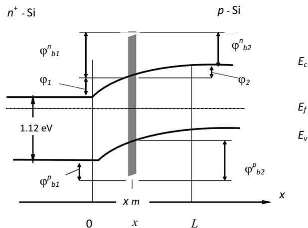
**Fig. 1.** Energy diagram of a  $p-n$  junction with a modified layer in its space charge region in the equilibrium state
