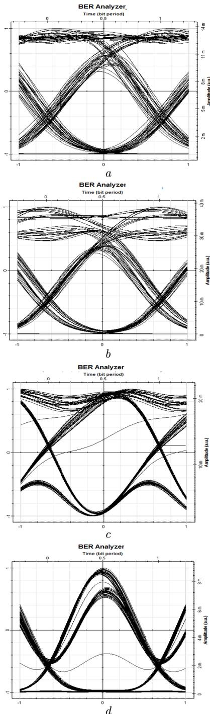
**Fig. 11.** Optimum eye diagram performance at 40 Gbps for 4 types of modulation formats at RZ-FSK (at BER =  $2.83 \times 10^{-18}$ ) (a), NRZ-FSK (at BER =  $5.94 \times 10^{-19}$ ) (b), DPSK (at BER =  $4.56 \times 10^{-68}$ ) (c) and Duobinary (at BER =  $2.51 \times 10^{-21}$ ) (d)
