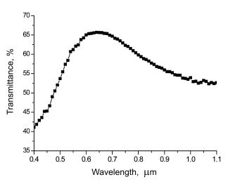
Fig. 3. Spectrum of light transmission through a glass substrate covered with a  $Cu_xS$  layer at the normal light incidence
