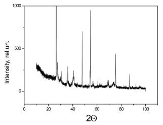
Fig. 1. X-ray diffraction spectrum of a CdS film
