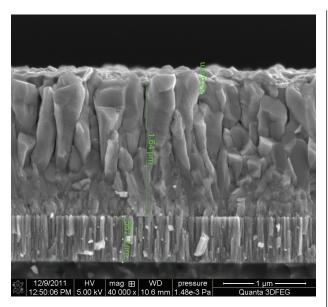
Fig. 2. Microscopic image of a cleaved facet of the CdS/CdTe/Cu<sub>x</sub>S structure
