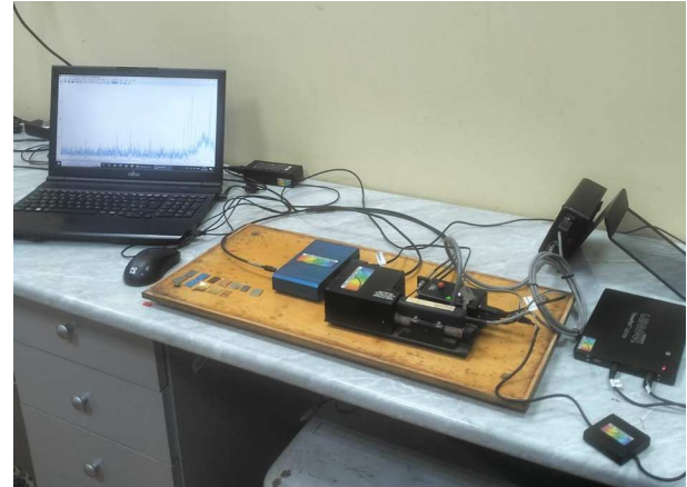
Fig. 1. StellarNet Blue-Wave (200–400 nm) spectroscopic system for LIBS and absorption measurements: laser–target interaction, optical fiber collection, and spectrometer-based detection
