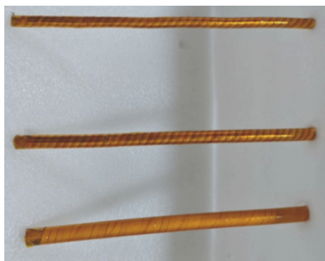
Fig. 11. Device output: 6 mm, 8 mm, 10 mm SC cables
