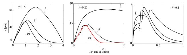
Fig. 3. I–V characteristics of contacts of lengths  $\mathcal{N} = 1, 9, 49$  (left and middle panels) and  $\mathcal{N} = 3, 5, 7$  (right panel) for different values of  $\gamma$  and  $\beta^{\text{cont}} = \gamma$ . The curve for N = 49 in the middle panel is marked with red color for clarity
