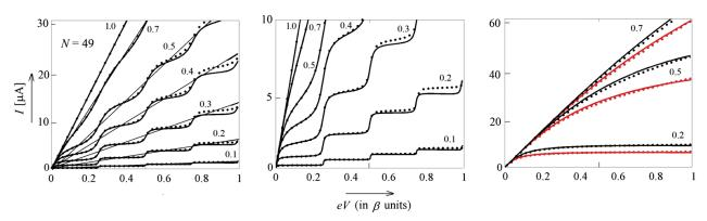
Fig. 4. Left panel: The exact dependence I(eV) given by Eq. (21) is depicted by solid lines while its approximation (22) is displayed by dotted lines calculated for  $\mathcal{N} = 49$ ,  $\beta^{\text{cont}} = 1$  and  $\gamma = 0.1$ , 0.2, 0.3, 0.4, 0.5, 0.7, and 1.0. Central panel: Enlarged dependences shown in the left panel. Right panel: The same dependences for N = 3 (black), N = 5 (red), and  $\gamma = 0.2$ , 0.5, and 0.7
