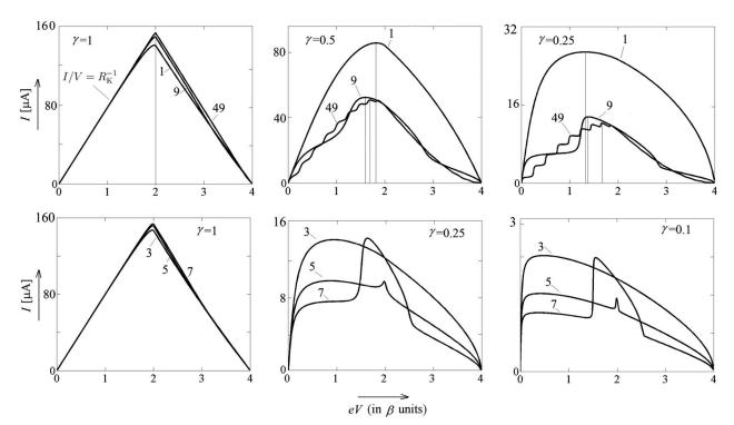
Fig. 2. I–V characteristics of contacts of lengths  $\mathcal{N} = 1$ , 9, 49 (top panel row) and  $\mathcal{N} = 3$ , 5, 7 (bottom panel row) for different values of  $\gamma$  and  $\beta^{\text{cont}} = 1$ . The left side of perfect isosceles triangle ( $\mathcal{N} = 49$ ,  $\gamma = 1$ ) corresponds to the volt-ampere characteristic  $I = \frac{2e^2}{h}V$ ,  $h/(2e^2) = 12.9k\Omega$
