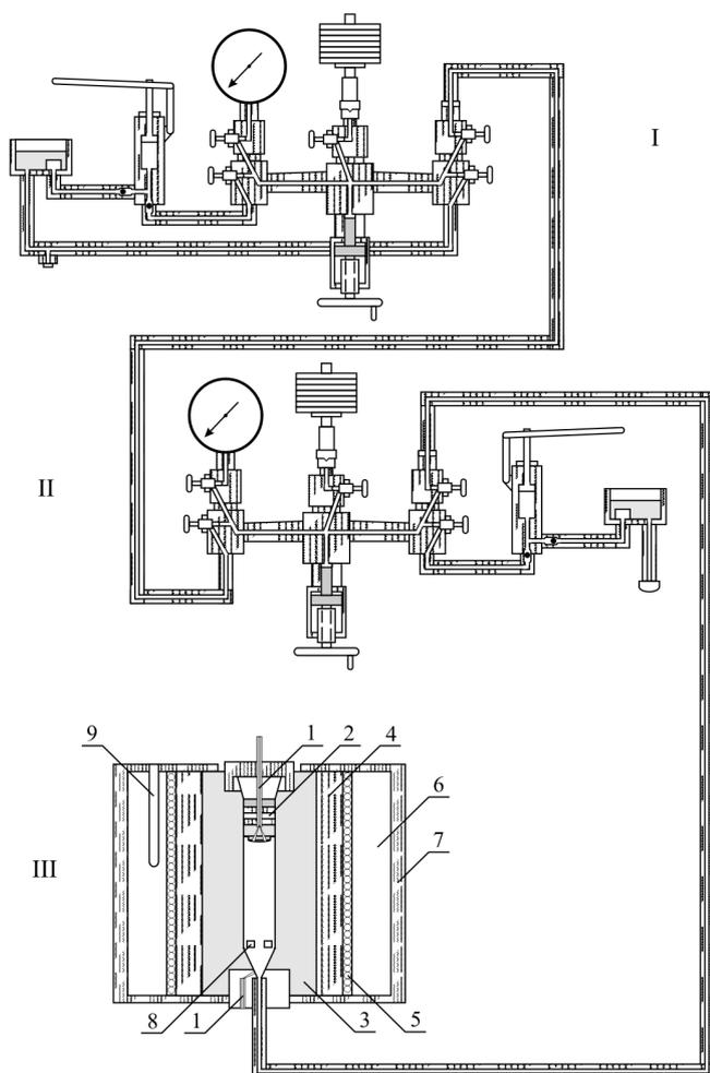
Fig. 1. Block diagram of the installation for  $P$ - $V$ - $T$  researches in liquid systems: (1) working chamber core, (2) sealing system, (3) high-pressure autoclave, (4) outer shell of the high-pressure autoclave, (5) electroheater winding, (6) fiber glass, (7) protection cell, (8) resistance thermometers, (9) cuvette for a thermometer
