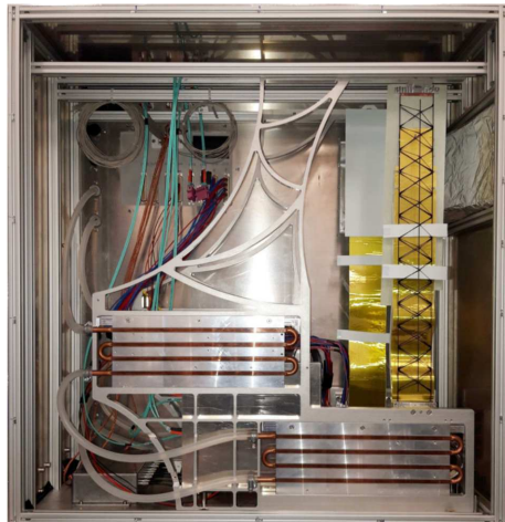
Fig. 7. mSTS detector modules mounted on the C-frames. Microcables running along the ladders and integrated cooling plates are visible
