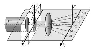
Fig. 5. Basic optical scheme for the correlation technique with periodic structures based on the "equivalent" interference pattern. The input plane wave is  $I^{\rm inp}$ , the equivalent phase mask is  $M_1$ , i.e. this is an additional phase grating with determined phase profile. The diffraction grating and the equivalent mask have either equal periods or multiple periods. The other designations are the same as in Fig. 1
