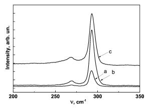
Fig. 1. Raman spectra of GaAs specimens: raw (a), No. 1 (b), and No. 4 (c). See Table for the specimen nomenclature
