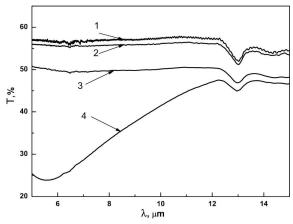
Fig. 3. IR transmission spectra of Cr-doped GaAs specimens [2]: (1) raw specimen, (2) specimen 1 after the HF treatment under a mask (a discharge power of 250 W, a gas pressure of 0.8 Torr, a treatment time of 15 min), (3) specimen 2 after the HF treatment under a mask (a discharge power of 250 W, a gas pressure of 0.8 Torr, a treatment time of 47 min, (4) specimen 3 after the annealing at 600 °C for 30 min in the argon atmosphere
