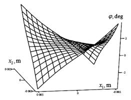
Fig. 3. Distribution function  $\phi(x_1, x_2)$  of the light-beam polarization plane rotation angle over the position of a light beam on the surface of the bimorphic element at the resonance frequency for the fundamental vibration mode
