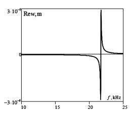
${\it Fig.~2.}$  Dependence of the real part of the bending function w at the center of a bimorphic plate on the linear resonance frequency for the fundamental mode of magneto-mechanical vibrations
