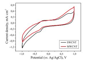
Fig. 3. CVs recorded for a queous SWCNT and MWCNT suspensions (1.0 KCl) on a GC electrode (0.24  $\rm cm^2)$  at v= = 0.10  $\rm V\cdot s^{-1}$
