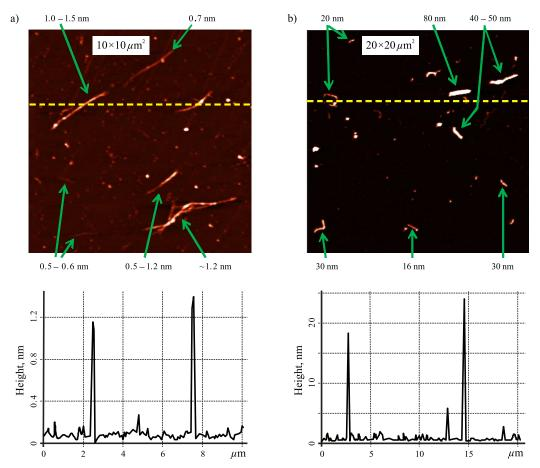
Fig. 2. AFM images of SWCNTs (a) and MWCNTs (b) deposited from an aqueous suspension (concentration: 5  $\mu$ g/ml) on the mica substrate (tapping mode). Topographic images for a given profile (dashed line) are shown on the top. The diameters of some CNTs are indicated by arrows
