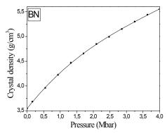
Fig. 10. Crystal density versus the hydrostatic pressure
