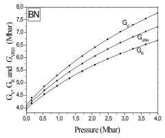
Fig. 3. Reuss modulus  $G_{\rm R}$ , Voigt modulus  $G_{\rm V}$ , and the shear modulus  $G_{\rm VRH}$  versus the hydrostatic pressure
