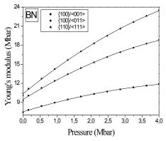
Fig. 7. Young modulus versus the hydrostatic pressure
