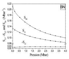
Fig. 6. Compliance constants  $S_{ij}$  versus the hydrostatic pressure
