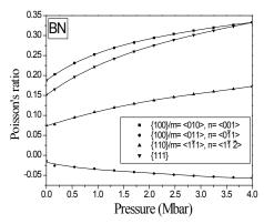
Fig. 8. Poisson's ratio versus the hydrostatic pressure
