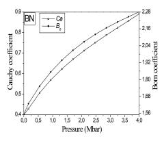
${\it Fig.~5.}$  Cauchy and Born coefficients versus the hydrostatic pressure
