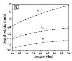
Fig. 11. Longitudinal, transverse, and average sound velocities in BN versus the hydrostatic pressure
