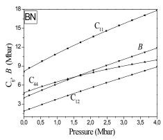
Fig. 1. Elastic stiffness constants  $C_{ij}$  and the bulk modulus B versus the hydrostatic pressure on (B3) BN
