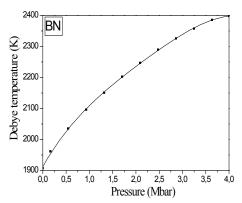
Fig. 12. Debye temperature versus the pressure
