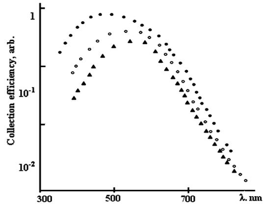
Fig. 5. Dependences of the collection efficiency on the incident light wavelength for solar cells with the Schottky barrier ( $\blacktriangle$ ),  $n-i-p$  heterojunction ( $\circ$ ), and double heterojunction ( $\bullet$ )
