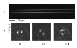
Fig. 2. Luminescent tracks and the transverse intensity distribution at a distance of 1.5 mm from the output face of the specimen excited with coaxial OV and vortex-free beams. The pulse energy in each beam equals 2  $\mu$ J
