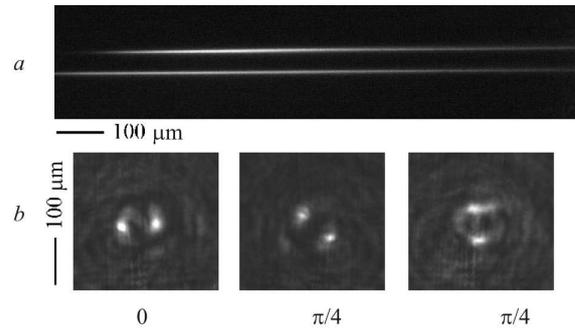
**Fig. 2.** Luminescent tracks and the transverse intensity distribution at a distance of 1.5 mm from the output face of the specimen excited with coaxial OV and vortex-free beams. The pulse energy in each beam equals  $2 \mu\text{J}$
