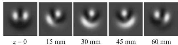
**Fig. 3.** Results of numerical simulation for the interference between an optical vortex with the topological charge  $l = 2$  and a plane wave. The length of each fragment side equals  $150 \mu\text{m}$
