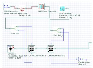
Fig. 3. Transmitter design for DPSK
