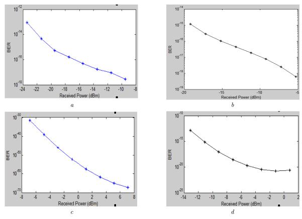
Fig. 10. BER as a function of the received power: RZ-FSK (a), NRZ-FSK (b), DPSK (c) and Duobinary (d)
