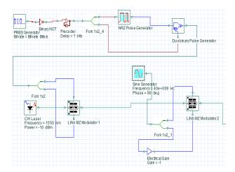
Fig. 4. Transmitter design for the duobinary modulation format
