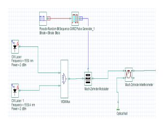
Fig. 2. Transmitter design for NRZ-FSK
