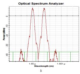
Fig. 8. Optical spectrum after 60 km for (a) DPSK at Pin = -16 and (b) Pin = -2 dBm
