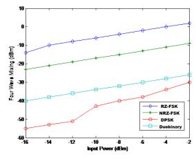
${\it Fig.~5.}$  Relationship between the FWM power and the input power at different modulation formats
