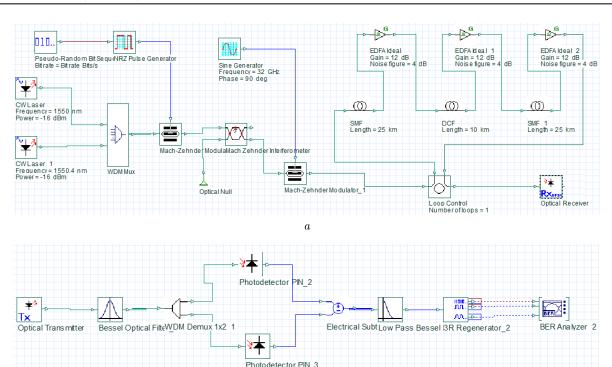
Fig. 1. System design for a RZ-FSK (a) transmitter and (b) a receiver
