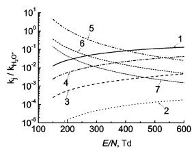
Fig. 4. Rate constants for ion generation in the water vapor discharge normalized by the rate constant for ion  $\rm H_2O^+$  generation as functions of E/N for various positive and negative ions:  $\rm OH^+$  (1),  $\rm H_2^+$  (2),  $\rm O^+$  (3),  $\rm H^+$  (4),  $\rm H^-$  (5),  $\rm O^-$  (6), and  $\rm OH^-$  (7)
