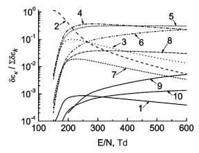
Fig. 5. Dependences of the energy losses of electrons at their collisions with water molecules on E/N
