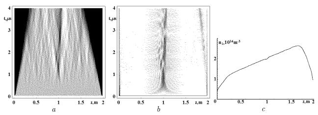
Fig. 2. Space-time distributions of ion density perturbations (a) and the electric field magnitude (b) and the spatial distribution of the ion density at the time moment  $t = 3 \ \mu s$  (c) for  $j_m = 0.03 \ mA/cm^2$
