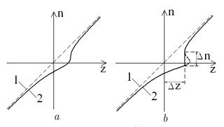
**Fig. 1.** Initial plasma density profile (1) and a stationary profile formed by the electric field excited by the given modulated beam current (2): a – beam current amplitude is less than the threshold value, b – beam current amplitude exceeds the threshold value (8). The coordinate origin corresponds to the local plasma resonance point of the initial density profile
