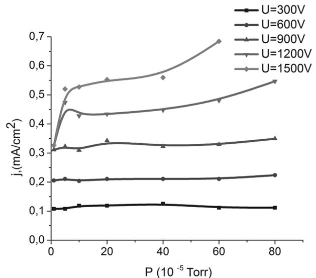
Fig. 2. Dependences of the discharge current density on the working gas pressure for various voltages across a discharge gap in the low-current mode
