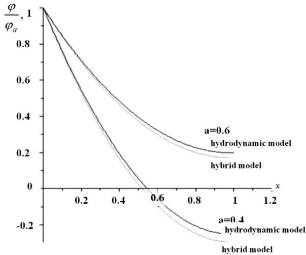
**Fig. 7.** Comparison between the results of numerical calculations for the potential distribution in the discharge gap in the hydrodynamic and hybrid models
