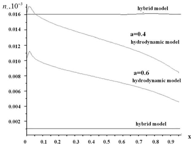
**Fig. 8.** Comparison between the results of numerical calculations for the electron concentration in the discharge gap in the hydrodynamic and hybrid models
