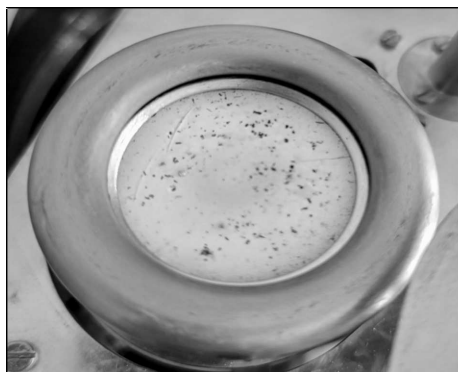
Fig. 1. Photo of GZO target for RF-magnetron sputtering
